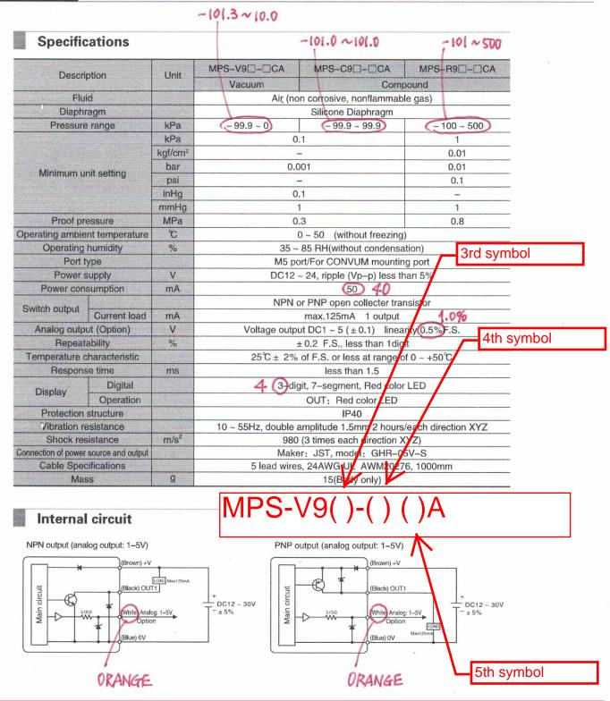
MPS-9A series is Analog output type only.
